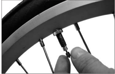
Before pumping up the tire, you have to unscrew the little knurled nut on the valve.
