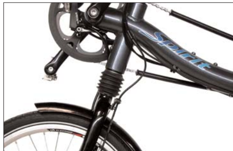
The suspension of the front wheel is integrated in the steering tube.
