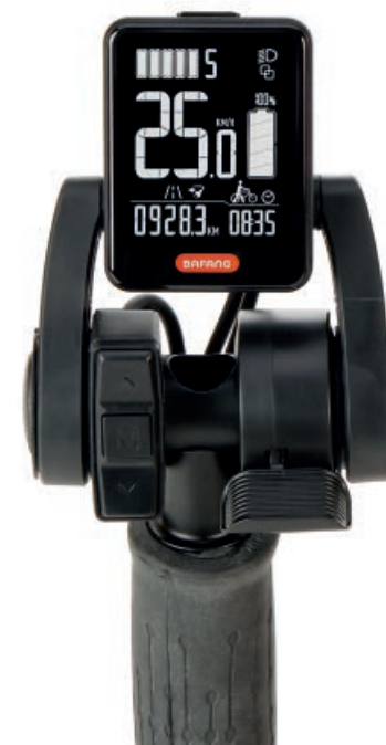
Below the display on the left are the touch buttons for switching the assistance level. Below the display on the right is the thumb throttle for extra power.
