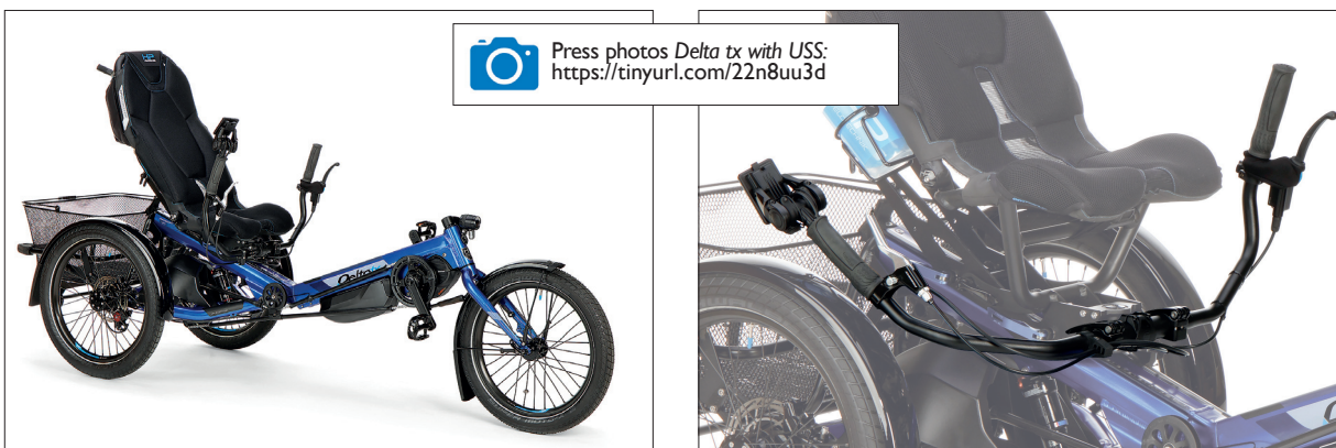
The Delta tx e-trike with Under Seat Steering. Right image: For even easier access, the handlebar can be folded away. Photos: HP VELOTECHNIK
