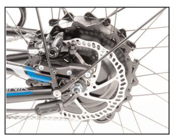
Figure 1: rear wheel with GO SwissDrive motor
