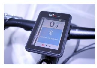
For connection of a compatible mobile telephone, the Bluetooth interface must be activated. The EVO operating element must be switched on via the "Bluetooth" sub-menu using the "Activate Bluetooth" button.
