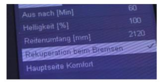
Note that the tyre circumference is a fundamental requirement for many calculations, such as the displayed speed and also the distance travelled and the distance remaining. If possible, have these settings changed by your specialist dealer before collecting the E-Bike.
