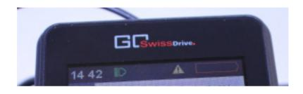
Battery charge level: The battery symbol on the right edge of the status line indicates the current charge level of the battery. The symbol has 9 bar segments with each bar representing 10% of the battery capacity. A detailed description of the display depending on the charge status can be found in the following table.
