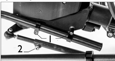
Leg rest: setting the inclination
