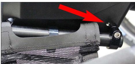
Leg rest: setting the inclination
