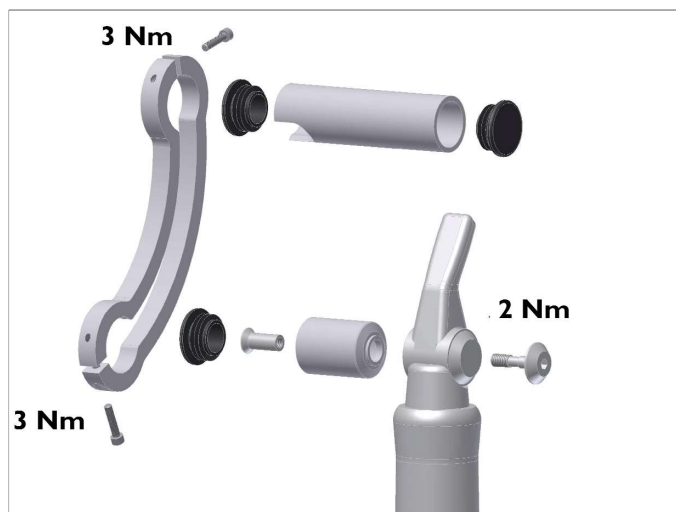
Fig.3: Mounting on a barend shifter MICROSHIFT BS 09 or STURMEY ARCHER HSJ 963
