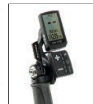
Right: On the under seat-steered Streetmachine Gte, the "Top View" mounting at the handlebar end can be used to bring the display closer to your field of vision, but slightly reduces the space available to mount the bike. Alternatively, it can be mounted next to the handlebar handle (picture bottom left).
