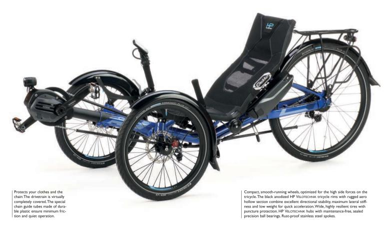
Wider is better: The wider the track width, the higher is the tilt stability and the faster your trike is when cornering. For this purpose the broad track of 78 cm (30%") of the Gekko fx 26 provides a lot of room between the wheels for your hands on the wide handlebars, allowing much wider steering angle for a small turning circle. To enable your trike to slip casually through doors and gates, HP VELOTECHNIK has developed narrow hubs for a low total width of only 83 cm (3½").
