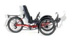
The Gekko fxs is based on the company's tried-and-tested design with its two characteristic front wheels. This design technique, referred to as tadpole-design by trike experts, is famed for its riding stability especially when a rider brakes during hard cornering. HP VELOTECHNIK design at its best: The frame is based on a main tube that holds the bottom bracket boom and it ends under the
