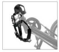
Pedal with heel strap: The alternative for those who do not want or may not be able to use SPD\* system pedals. Easy entry with any kind of shoe through the automatically self-righting positioning. One hand tightening allows for safe and efficient pedaling. One grasp is enough to release the shoe again when needed.
