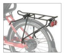
The stable Rear rack for two panniers up to a 25 kg (55 lbs) load is optimal for the high lateral forces when riding a tricycle. Your panniers ride low and close to the rider. next to the rear wheel. The advantage of the Gekko series: The platform for larger panniers is already integrated above the rear wheel. The rack is made of aluminum tubes (10 mm / 0.39") with black powder coating.
