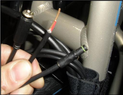
left: wire with DC plug for recuperation switch
