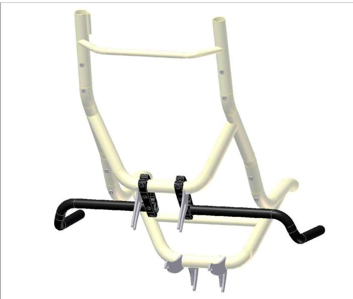
Fig. 5: For Ergomesh seat HS XL: Installation of the frame clamps between the seat supports. The frame clamps can also be mounted on the frame under the seat (compare fig. 4) between the seat brackets.
