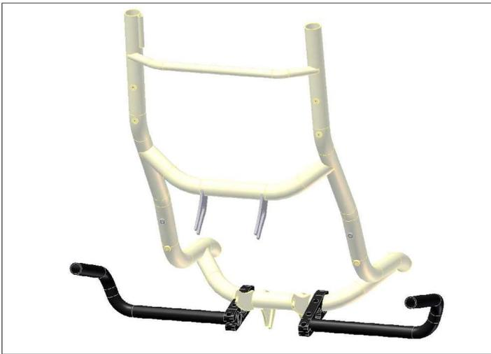
Fig. 4: Mounting the frame clamps on the frame under the seat with the holder tubes facing upwards and backwards.
