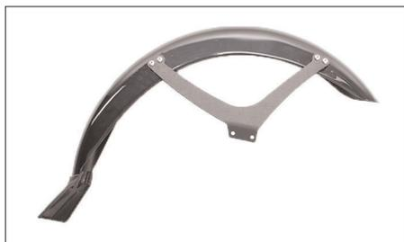
*Position of the mounting bracket in respect to the mudguard (left side part)*
