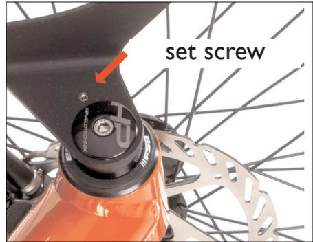
Put on the A-head cap and insert its screw. To adjust the headset, refer to the trike's operating manual.
