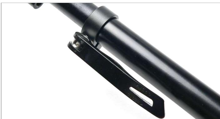
17. To compensate for settling, open and close the two quick release levers several times and then check the prescribed tightening torque of the screws again.
