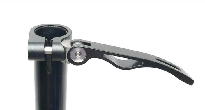
15. Slide the stem upper part with handlebars into the stem middle part and close the quick release. Use a friction-enhancing assembly paste in the clamping area (e.g. DYNAMIC Carbon paste).
