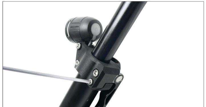
24. Screw the cable guide back onto the stem middle part.
