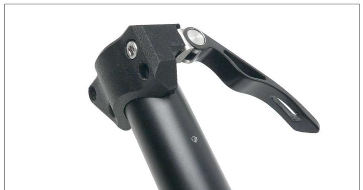
11. Screw the M3 screw completely through the light- and cable holder into the clamp using medium-strength thread-locker (e.g. Loctite 243) and tighten it to 1 Nm. Make sure that the screw does not protrude into the lower stem part so that the stem middle part is not damaged when it is pushed in.
