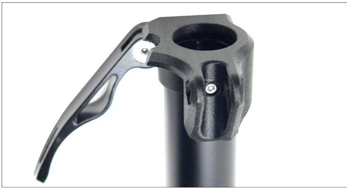
12. Push the stem middle part back into the lower stem part and close the quick release.
