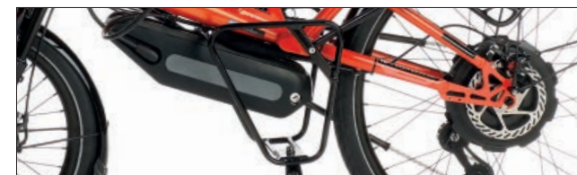
Top: The battery is ideally placed in the middle of the bike under the seat with a low center of gravity. All HP VELOTECHNIK recumbents with Above Seat Steering offer space for this, the Streetmachine Gte also with Under Seat Steering. The lockable battery can be easily removed for charging.
