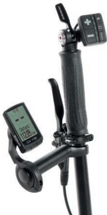
Easy-to-read 2.4-inch display, mounted here beside the handlebar grip.
