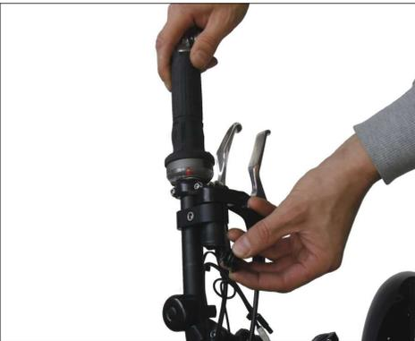
8) Before the first ride make sure both brake levers can be operated safely and that they do not interfere with the steering.
