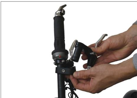
**⚠ Danger!** Before the first ride check that both brake levers are securely fastened, operatable and the steering is fully functionable. A faulty braking system or steering may lead to serious crash and injury!
