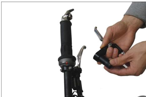
3) Tighten the clamp of the additional brake lever using the torque specified by the brakelever manufacturer. Put in the bar end plug.
