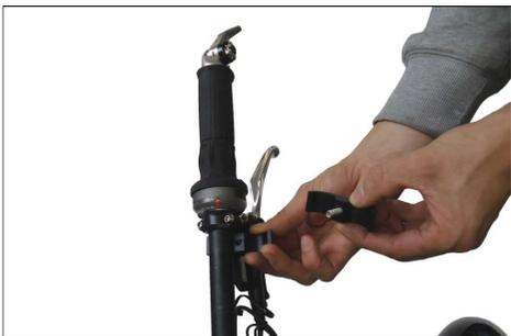
5) Slide the tube with the brake lever into the clamp from above. Position the clamp and the brake lever according to your needs.
