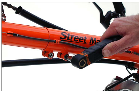
Unscrew the clamping screw to adjust the front boom.
