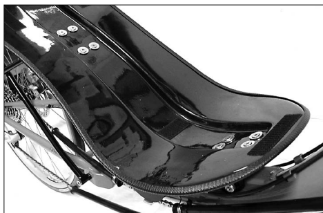
HP VELOTECHNIK's seats feature a special channel for the spine. You can individually adjust the padding.
