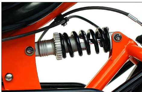
Suspension element DV-22 with fixed damping rate.
