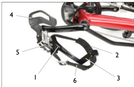
Heel support sheet (1), heel support strap tube (2), heel support hook (3), pedal toe clip (4), pedal (5) and heel support strap (6)
