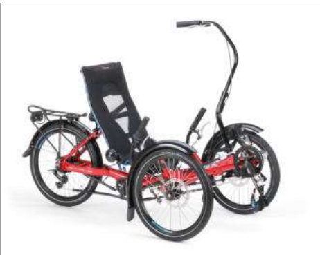
The solid companion bar on the Gekko fxs enables ermöglicht co-steering, accelerating and active braking
