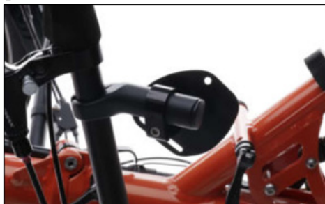
Attachement bolt M5 x 16 of pivotal clamp
