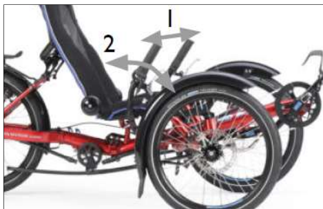
The handlebar allows adjustment in width (1) and angle (2)
