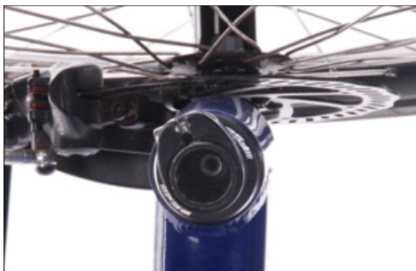
View into head set with star fangled nut inside
