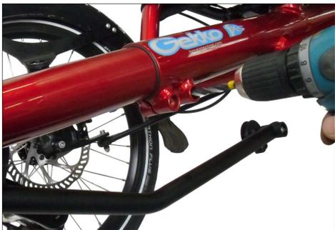
**11)** Slide both M6 inside threaded sleeves from the left side into the eyelets. There is a 5 mm hex wrench socket in one side of the sleeves which must face outwards.
