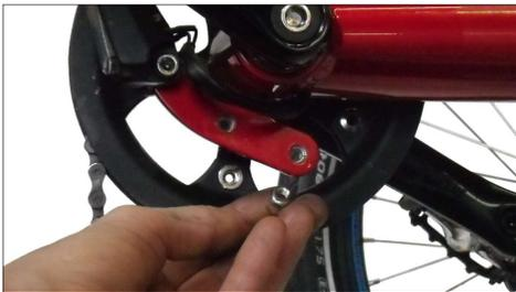
With front booms for Shimano STEPS assistance systems an adapter bracket must be mounted first, using the included countersunk screws. Don't use set nuts to mount the pulley tube. Threads are already included in the bracket.
