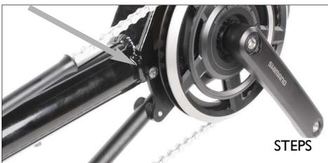
**6)** Tighten the screws gently at first. The set nut's collar is pulled into the material of the bracket and prevents the nut from turning.
