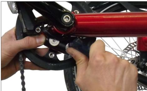
**9)** Remove both bolts from the front boom clamping.
