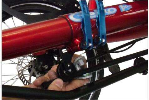
**17)** Guide the chain around the pulleys and reconnect the chain ends. You may have to add spare chain in order to reach the correct chain length.
