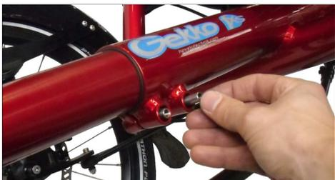
**12)** From the right side mount the sheetmetal bracket with mushroom-head screws and washers under the screw head. The mounted pulley faces forward and down. Slide the bracket as much forward as possible in its long holes.
