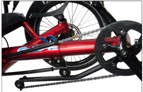
**19)** Check the screws of the pulleys for being tight enough (tightening torque ca. 6 Nm).
