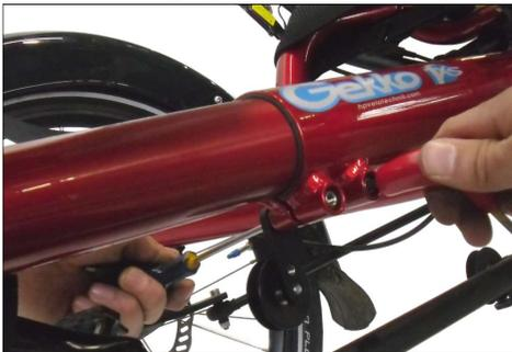
**14)** Mount the bushings, springs, calottes and quick releases in the order shown in the picture below.
