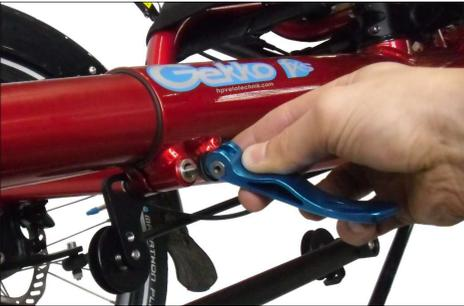
**⚠ Danger!** Both quick release levers must be firmly closed before riding. Lever force 15 – 20 kg (33 – 44 pound). Not properly closed quick releases allow the front boom to turn while riding. Danger of accident!
