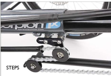
**13)** Tighten the mushroom-head screws. Use a 5 mm hex wrench on the threaded sleeves to prevent them from turning. Tighten to 9 Nm.
