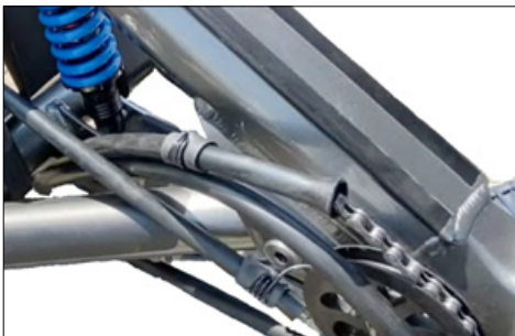
Slide the chain between the swingarm's tubes.
