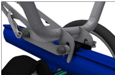
Right side (in direction of travel) of the mounted seat adapter with seat frame. The blue lever is shown in light gray in the picture.
