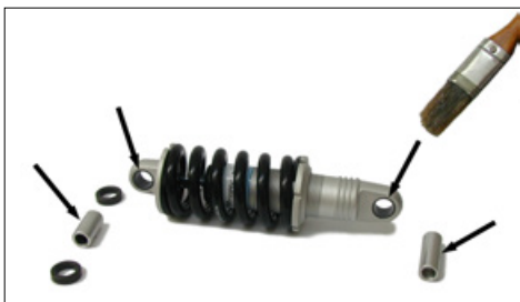
The bushings of the rear spring element need to be lubricated
