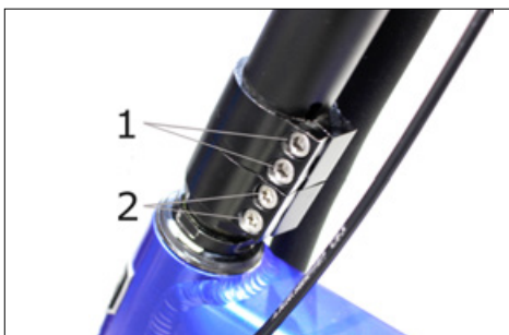
1 - Allen screws to secure the stem on the fork. 2 - Torx screws for the fork clamping
