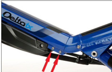
The M6 screws clamp the frame.
