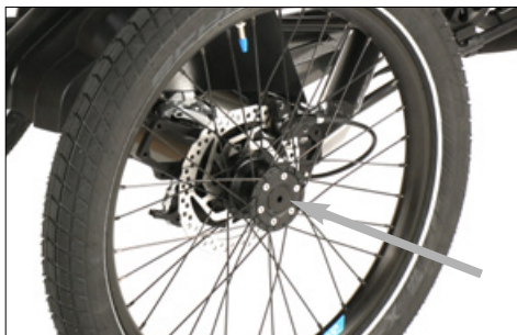
The central bolt needs to be opened.
