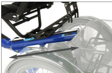
The seat adapter can be slid on the rear frame for adjustment
