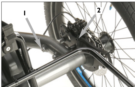
Brake support sheet screws (1) and caliper mounting screws (2)
