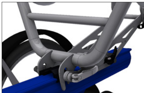
Left side (in direction of travel) of the mounted seat adapter with seat frame. The quick-release clamp with blue lever (shown in light gray in the picture) is used to attach both the seat to the seat adapter and the seat adapter to the seat rail.
