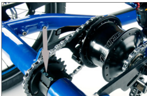
When dismantling the right rear wheel or mounting the left rear wheel: Use a chain whip to fix the axle mounted sprocket.
