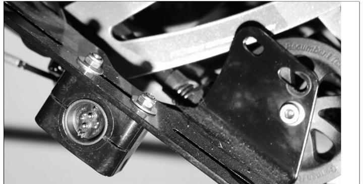
Rosenberger socket mounted on a battery adapter
