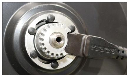
Insert the plug of the motor cable into the respective socket on the motor.
