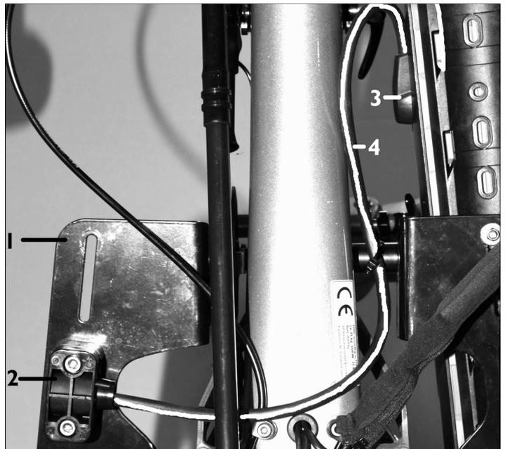
Cable routing between the Rosenberger socket and the battery mounted on the left side, seen from the underside of the trike.
