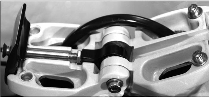
HP VELOTECHNIK plug-in cable harness routed through the folding hinge
