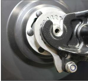
Place the rear wheel in the dropouts so that the torque retainer engages in the support screw.
