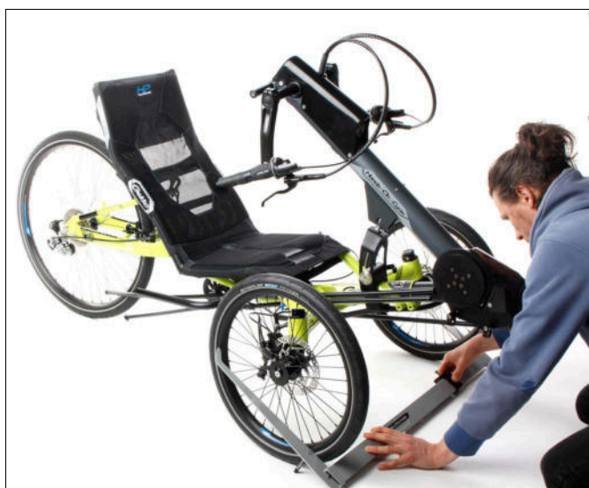
Fig. 42: Adjust the toe-in
