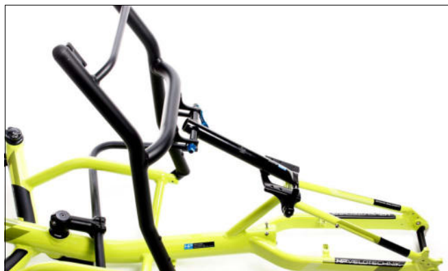
Fig. 2: Mount the HP VELOTECHNIK assembly mount between frame and seat frame.
