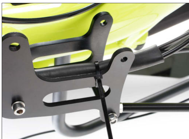
Fig. 24: Guide the cable harness between lower stem and stem adapter. If necessary, move the protective tube so it protects the cable harness from the stem adapter's edges. Fixate it with a zip tie (in the picture: Gekko 26).
