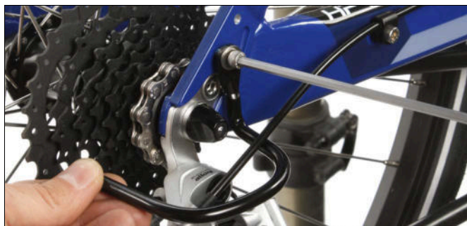
Fig. 16: Rear derailleur protection (only for Gekko fx 26, picture shows a different equipment)
