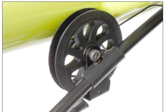
Fig. 35: the chain protection tube is mounted to the chain tube holder metal
