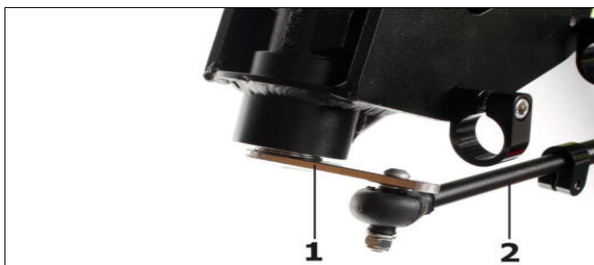
Fig. 28: Steering rod mounted at the steering lever 1 - steering lever 2 - steering rod
