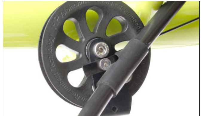
Fig. 34: Put the rubber sleeve onto the front edge of the chain tube holder metal and pull it rearwards.
