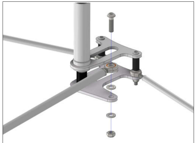
Fig. 26: Gekko 26 part order when mounting the steering rod to the stem adapter
