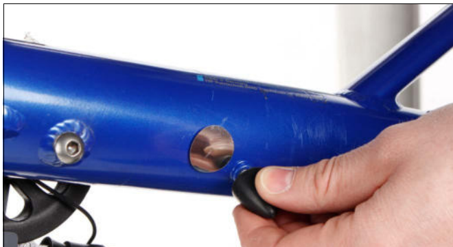
Fig. 36: Mount the stainless steel protection sticker and folding buffer (only Gekko fx 26).
