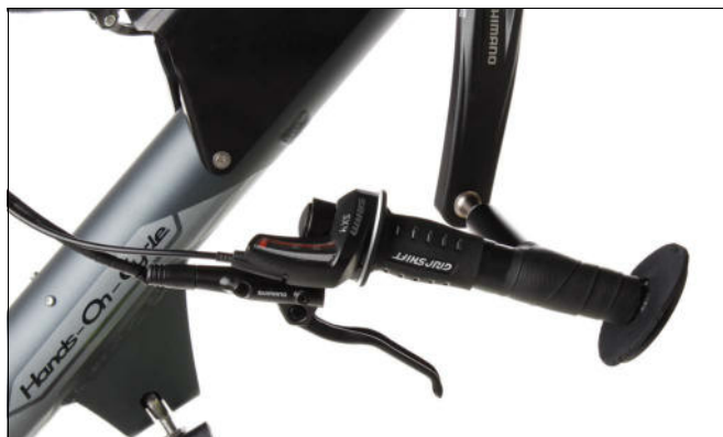
Fig. 30: Brake lever and gear shifter mounted on the hand pedal
