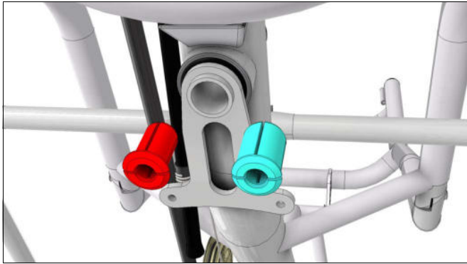
Fig. 20: Choose the correct adapter for the lower stem.
