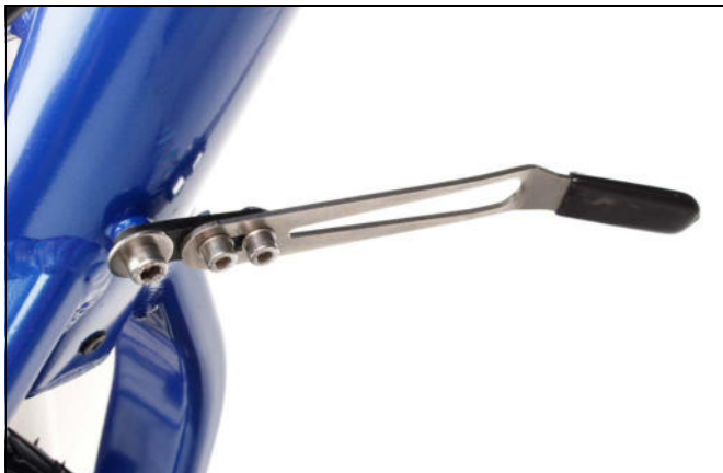
Fig. 38: Mounted folding lock plate with extension plate. (only Gekko fx 26)
