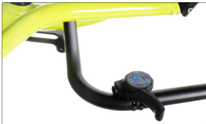
Fig. 17: Mount the parking brake actuation lever on the handlebar on the left side behind the bending.
