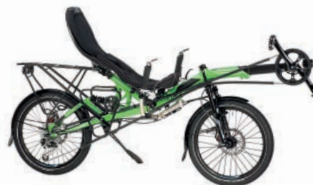
Grasshopper fx: Fast folding, fully suspended trekking recumbent with compact 20-inch rear wheel and medium seat height, ideal for smaller riders, from $ 4,990
