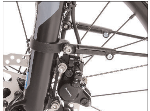
Attachment to the fork with a clamp, possible with Streetmachine and Grasshopper
