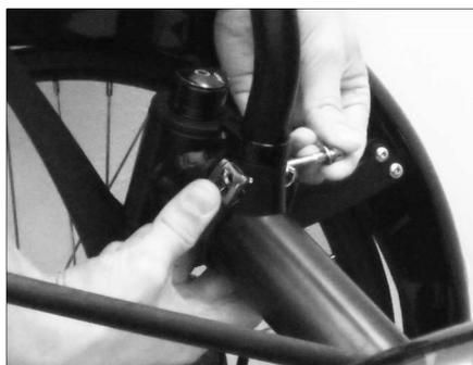
To fix the adapter, first use the longer cylinder head screw (45 mm) to preform the hose clamp. Then replace the screw with the shorter cylinder head screw (40mm), placing a washer under the screw head. Tighten the screw with a torque of 8–10 Nm.
