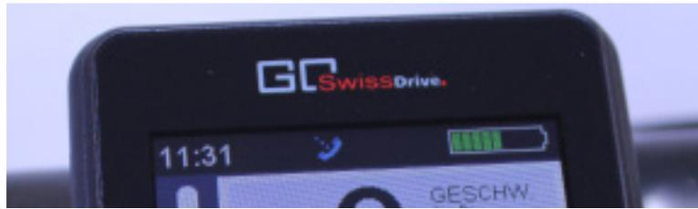
Fault: If a fault occurs in the GO SwissDrive drive system of the E-Bike, this is shown in the display. A pop-up appears (see chapter 7.2 "Warning notices") along with a fault symbol in the status line.
