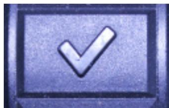
**[ + ]/[ - ] buttons:** The power assistance level of the GO SwissDrive drive system can be set with the [ + ]/[ - ] buttons. In the configuration menu, the [ + ]/[ - ] buttons are used to navigate between the individual menu items and change numeric values.
