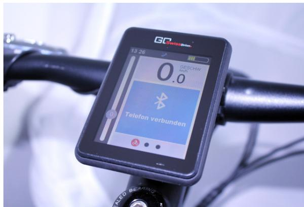
For connection of a compatible mobile telephone, the Bluetooth interface must be activated. The EVO operating element must be switched on via the "Bluetooth" sub-menu using the "Activate Bluetooth" button.
