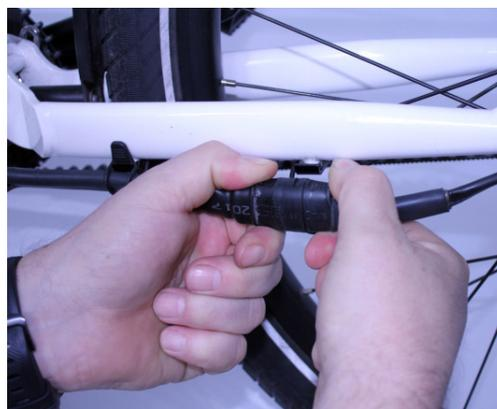
8. Finally, attach the cable with a cable tie or secure in the dedicated position on the frame. The cable should not protrude outwardly to the side nor interfere with the spokes of the rear wheel or rub against the motor.
