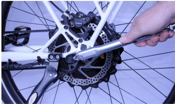
4. Tighten the torque arm bolts to the specified torque of 8-9 Nm to the frame.
