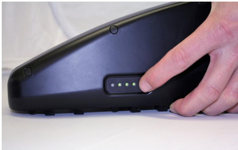
To ensure that the destination can always be reached with full power assistance and the battery service life is as long as possible, our recommendation is for the battery to be recharged after every long journey.
