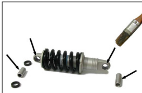
The bushings of the rear spring element need to be lubricated once a year.
