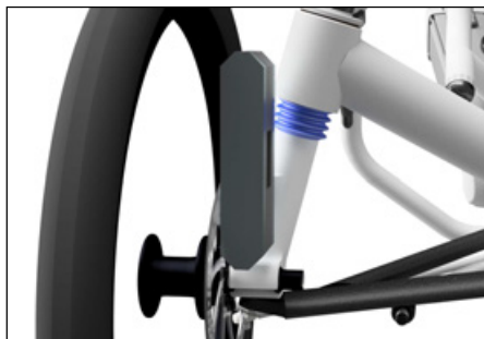
Align the protractor parallel to the brake disc.
