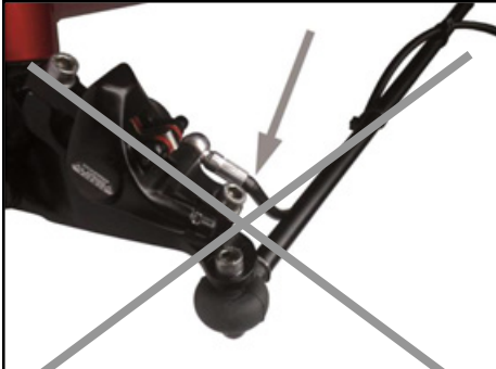
WRONG! The bow of the hose is routed under the track rod: Danger of snapping off the hose (cf. arrow).
