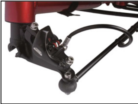
RIGHT: Lead the wire in a wide bow to the track rod. Check clearance when steering left and right
