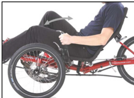
The handlebar angle is individually adjustable.
