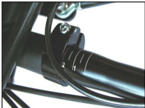
Handlebar width and angle are adjusted with the clamp at the stem under the main frame.
