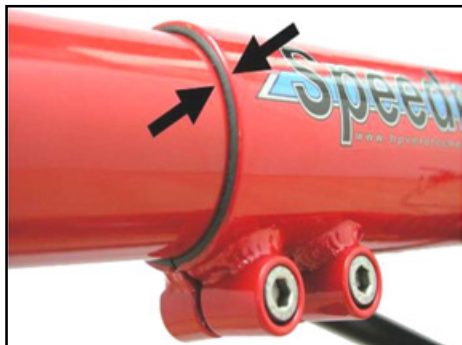
The plastic bush between front boom and main frame must be visible at all time.
