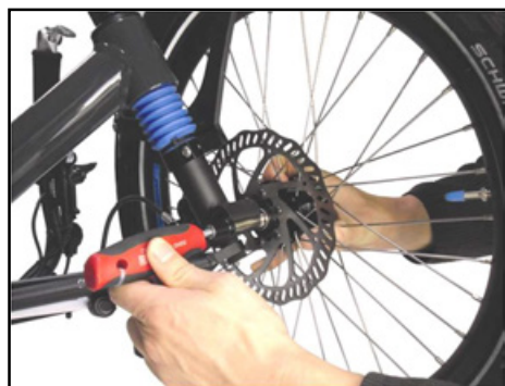
Loosen the screw in the locking part
