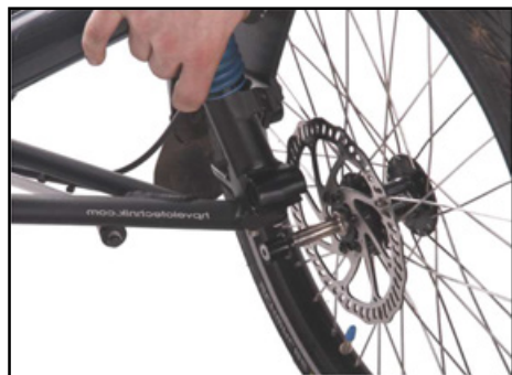
Taking out the front wheel out of the knuckle
