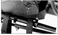
Fig. 9: The leg rest mesh is fixed in front of the clamps.
