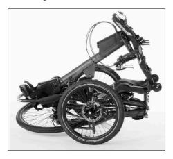
Fig. 1: Folded Gekko fx 26 with Hands-On-Cycle hand drive.
