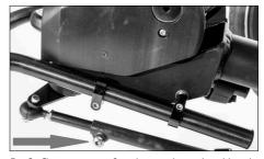
Fig. 3: Clamping screw for adjusting the push rod length
