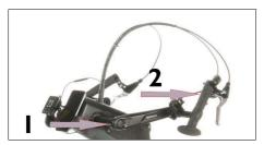
Fig. 12: Adjustments cranks and hand pedal I - Correct the distance between the cranks 2 - Shorten the hand pedal
