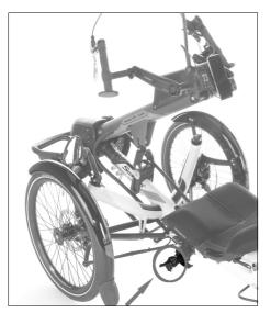
Abb. I: Parking brake: Move the lever forward to lock the parking brake. Move the lever back to release the parking brake.
