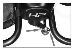
Fig. 13: For the attachment of the push rod and adjustment of the steering there are 2 threads on the steering lever to choose from.
