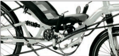
Comfortable ergo-bars under the seat for relaxed arms and wrists. Large steering angle through indirect steering. Maintenance-free bearings with sealed industrial bearings and self-lubricating rod ends.
