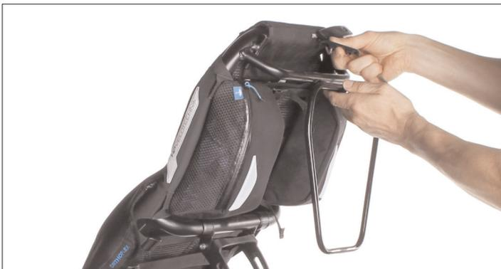
5. Screw the belonging screws loosely into the clamp.
