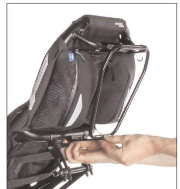
10. Place the upper part of the long clamp on the lower part from above. Prior to this, for ErgoMesh-Premium seats the other half of the clamping sleeve must be positioned in the large half-round of the clamp upper part.
