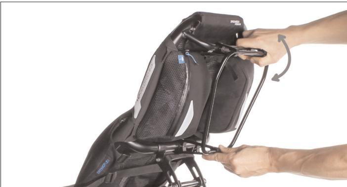
14. Tighten all screws with 7–9 Nm.
