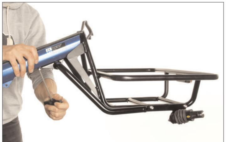
24. Pull the swingarm upwards and reconnect the damper with the main frame (tightening torque 6 – 8 Nm).
