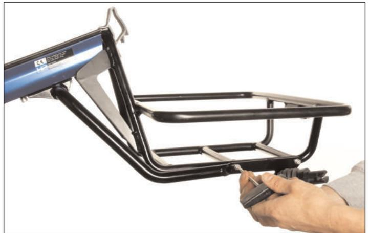
23. Tighten all connections of the stiffener arm with 7–9 Nm.
