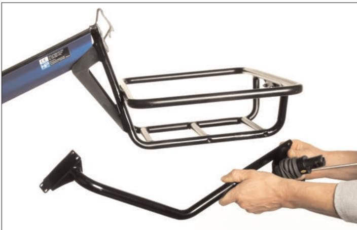
6. Connect the stiffener arm with the carrier by the rear hole of the carrier. Without anti-tilt wheels mounted, use a M6x20 screw with washer. With anti-tilt wheels mounted use a M6x30 screw with washer. Put the screw with washer through the stiffener arm, the sheetmetal bracket, and the curved plastic washer into the carrier's thread. Screw in the screw completely but do not tighten it.
