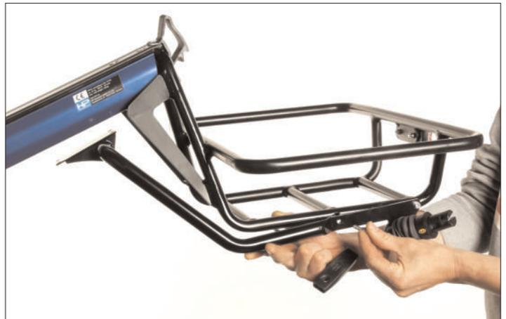
8. Turn the tricycle over so that the underside of the rear frame tube is accessible.
