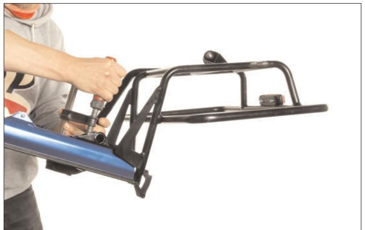
11. Drill the 4 holes in the sheetmetal through the frame tube wall using a 6,5mm drill.
