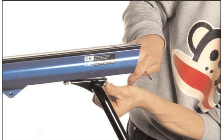
21. Reassemble the carrier and the retainer.
