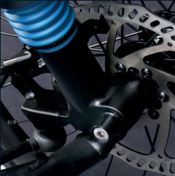
Lightweight aluminium wheel carrier with shock boot on the suspension strut. Blasted and black matte anodized finish. Housing gaskets over the tie rod's outer ball in the area of the wheels at risk from spray water.
