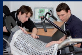
Computerized pressure distribution analysed on a BodyLink seat for the ideal shape.
