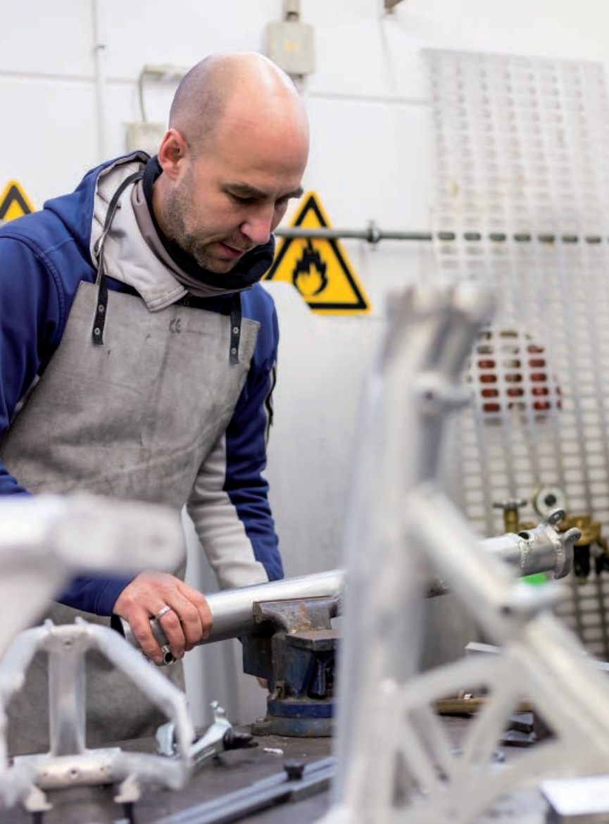
CEO Daniel Pulvermüller gets his hands dirty during prototype production. The series frames made of high-strength aluminum alloy are welded and heat treated by dedicated frame builders in partner factories.
