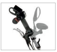
Everything from a single source: People who need all the controls on their bike on one side of the handlebars can choose the *One-hand operation* option: Thanks to custommade manufacturing, we can install engine control, gear shift, brake, plus parking brake and light with turn signals left or right.
