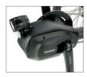
**By far the most affordable electric motor** in our modular system comes in a particularly small housing. This fits elegantly on the bottom bracket boom of your *Gekko*, which is specially forged for the *STEPS* motors.
