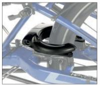
Immobiliser: Push out the handle, pull out the key - and the powerful AXA Frame lock effectively locks the rear wheel. The AXA accessory Chain for Frame lock (1 m / 39" long) is recommended as an extra to securely lock the trike.
