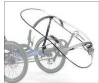
Protection against the wind and rain: The Streamer front cover from HP VELOTECHNIK keeps your feet warm and your legs dry. The cover's angle and height are adjustable. The cover can be easily removed using the quick release lever and rolled up for transportation. Teardrop-shaped for low wind resistance. Weight approx. 2.2 kg (4.8 lbs). Made of transparent, break-resistant plastic.
