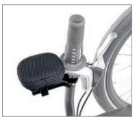
Hand rest: a real increase in comfort for all trike drivers. The hands steer lightly without having to support the weights of the lower arm. The comfortably padded hand rests can be individually adjusted to all angles and inclinations. Also available with a possibility to fixate the lower arm — an ideal add-on for the one-hand operation of brakes and drivetrain.
