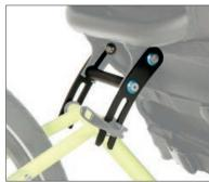
With the Seat Angle Adapter you can make the seat 9° steeper, but you can still vary the inclination (48° - 56°). Suitable for models Gekko fx 20, Gekko fx 26 and Gekko 26.
