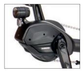
**Surprising:** The system is located in the mid-price segment, but is very powerful. A torque of 60 newton meters means an increase of 50 percent compared to the *E5000*.
