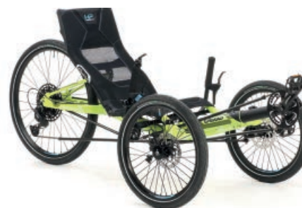
Gekko 26: Complete trike with rigid frame, raised seat position and 26-inch rear wheel, for rider size 1.60 – 2.00 m (5¼' – 6½') from € 3.190
