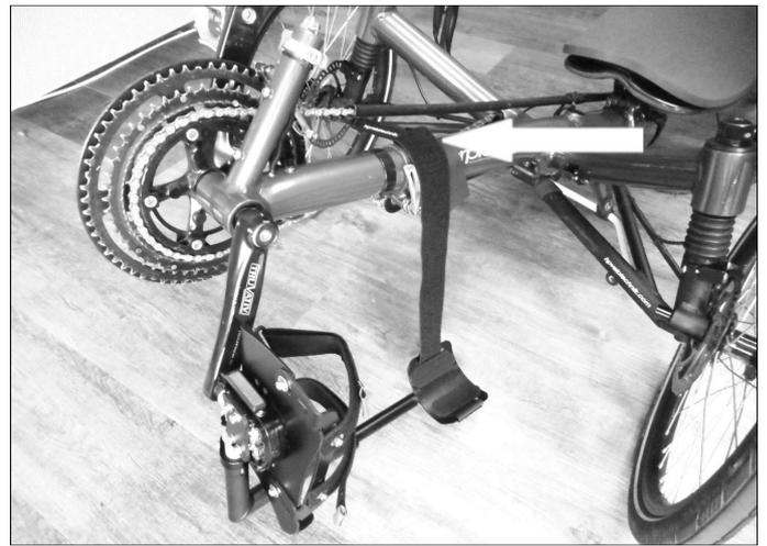
Fig. 7: Positioning of the Velcro strip to hold the lower leg fixation in place
