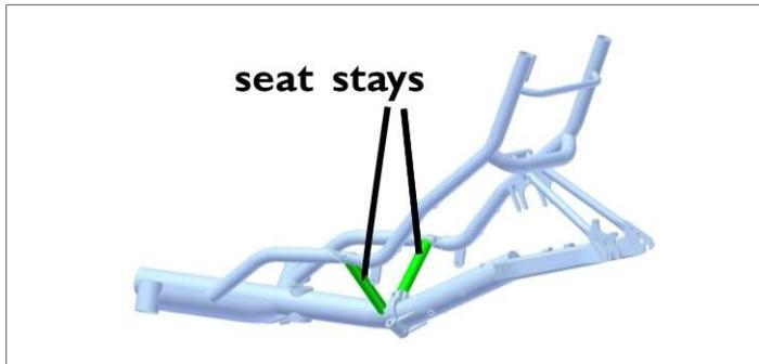
Fig. 3: The Side Bag Mounts are attached to the seat stays.
