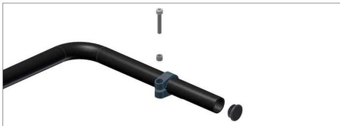
Fig. 6: Mounting of the clamp and end caps on the holder tube.
