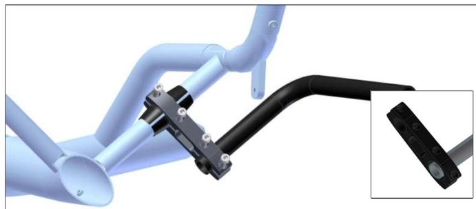
Fig. 4: Assembly of adapter sleeve, frame clamp and holder tube. View on the right seat stay from diagonally behind, the holder tube points to the rear wheel.
