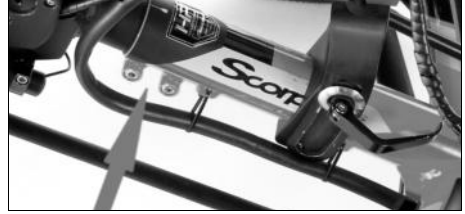
Abb. 2: Front boom adjusting clamp
