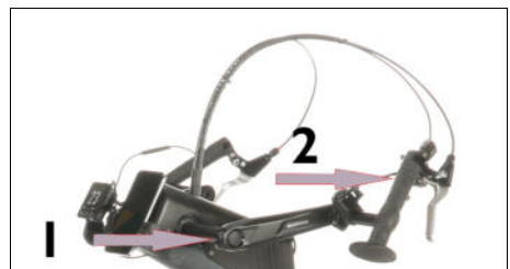
Fig. 11: Adjustments cranks and hand pedal 1 - Correct the distance between the cranks 2 - Shorten the hand pedal
