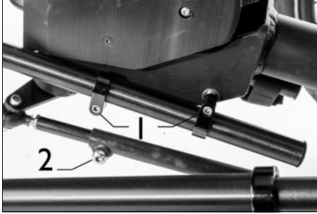
Fig. 7: 1 - Leg rest :adjustment of length 2 - push rod: setting of length.
