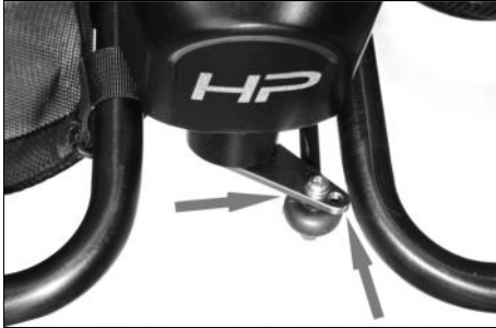
Fig. 12: For the attachment of the push rod and adjustment of the steering there are 2 threads on the steering lever to choose from.
