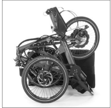
Fig. 2: Folded Scorpion fs 20 with Hands-On-Cycle hand drive. The seat was taken off.
