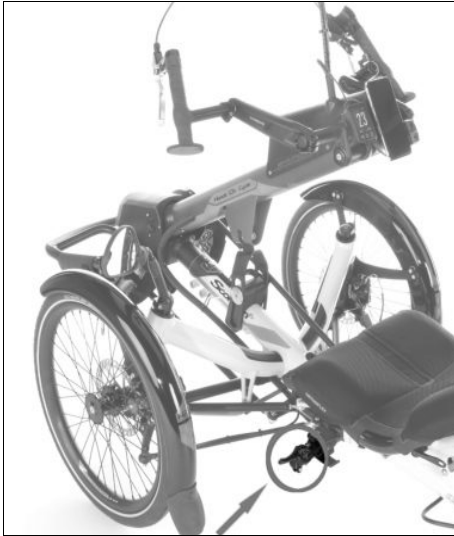
Abb. 1: Parking brake: Move the lever forward to lock the parking brake. Move the lever back to release the parking brake.
