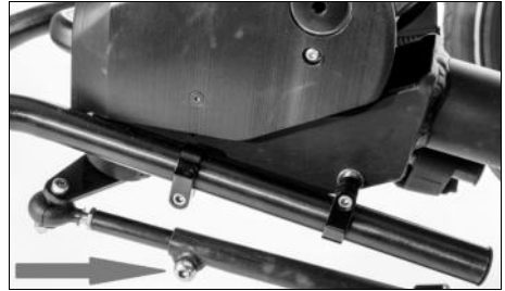
Abb. 3: Clamping screw for adjusting the push rod length
