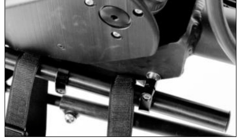
Fig. 8: The leg rest mesh is fixed in front of the clamps.
