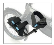
The ErgoPedal with calf brace is especially for users with functional impairments of feet and lower legs. This allows simultaneous active and passive movements which can mobilise with every turn of the crank. Angle. width and height of the lower leg support are adjustable. This version does not rely on an SPD® pedal for stability reasons.
