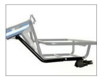
The optional *Trailer coupling* is designed for child or cargo trailers with WEBER coupling. Permissible towing capacity: 40 kg.
