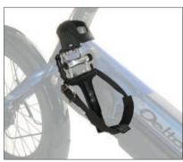
Pedal with heel strap: The alternative for all those who do not want to or cannot use clipless pedal systems. Easy entry with any type of shoe thanks to the automatically selfrighting positioning. Very firm hold, no accidental opening due to foot movement. To release the shoe, press briefly on the rubber reinforcement of the heel strap.
