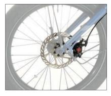
The Delta tx® is equipped with two independent brakes. It comes stock with separately controlled rear brakes. If you select the Coupled disc brake option, you will need an additional stopper. If you choose to have the additional brake mounted at the front wheel instead of the rear wheel, the splitting capability of your Delta tx® will be limited due to the cable routing.
