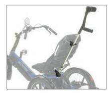
Walking aid mount: Easy insertion, safe transport and fast removal of walking aids. The practical fastener adjusts seamlessly to diameters from 20 to 31 mm (0.78" to 1.18"). HP VELOTECHNIK's stainless steel clip fixates the walking aid. To release, you can operate it with one hand.
