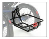
The Luggage rack made of sturdy 20 mm aluminum tubing carries 25 kg. It can also be used without the basket. If you also want to remove the rack when splitting the bike: remove it by loosening 3 screws and disconnect the plug connection to the rear light.
