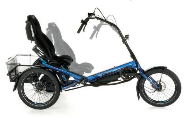
The main frame of the *Delta tx*® comes in one size. It offers space for people between 1.50 (4'9") and 2.00 meters (6'6") tall. For stepless adjustment, simply open the two quick-release levers to slide the seat on the upper frame railing.
